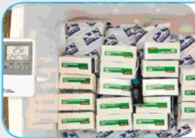
Place the thermometer probe with the top layer of vaccine.
